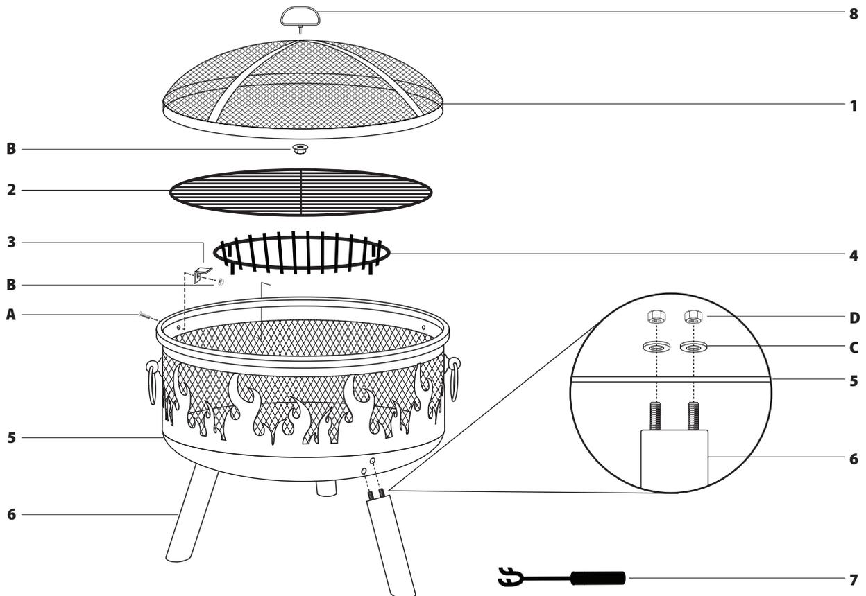
**STEP 1 - Attach 3 x legs (6) onto the outside of the firepit (5) by feeding the pre-attached thread through the holes**
